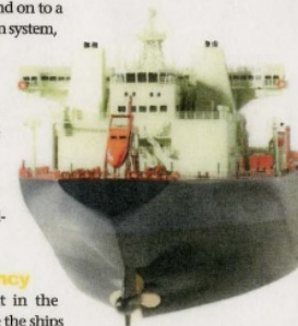
Stern view showing the ice cutting stern and the podded drive
